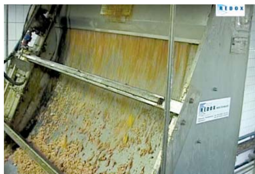
"Falling screen" separator to extract solids from effluent using gravity • kindly supplied by G & C Food Equipment
