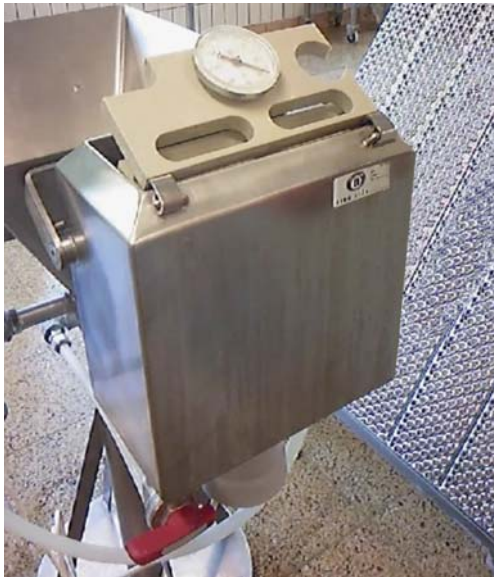
Knife steriliser, twin-walled to improve insulation and fitted element to heat water and visual temperature gauge
