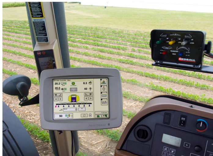
Figure 3.2 A typical sprayer control system using touch-screen control menus (from John Deere Ltd).
