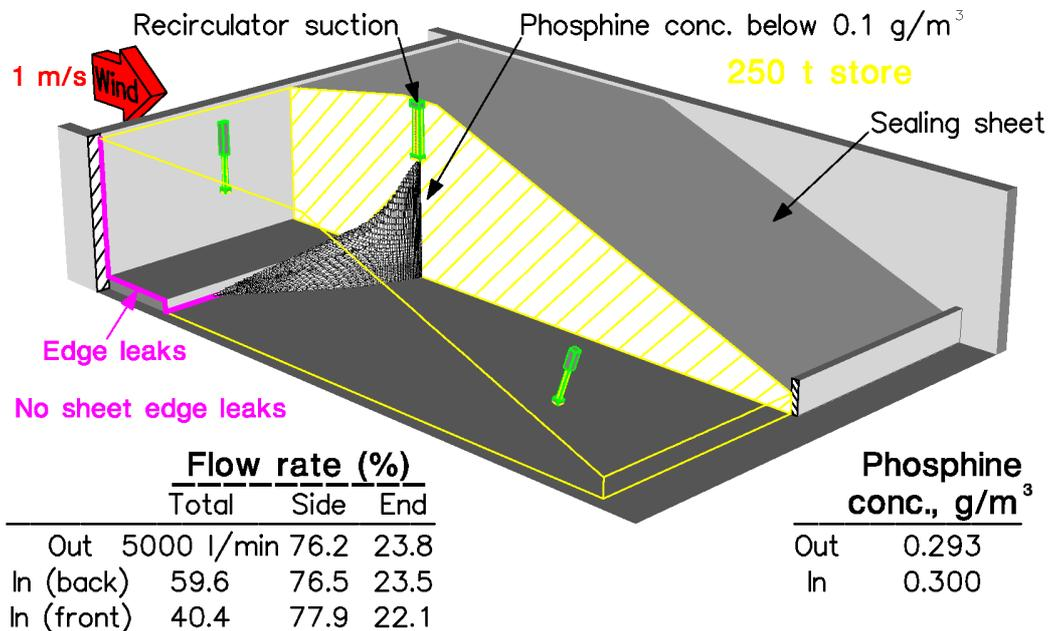
Figures 12 and 14 show that the effects of a  $1 \text{ m s}^{-1}$  wind blowing over the store have been included in the simulation. The pressures created by the wind were calculated in a separate model. The pressures at the leaks, relative to a downstream datum, were less than  $0.5 \text{ Pa}$  and the predicted effect of a modest wind on leakage rates when the system is running is negligible.
