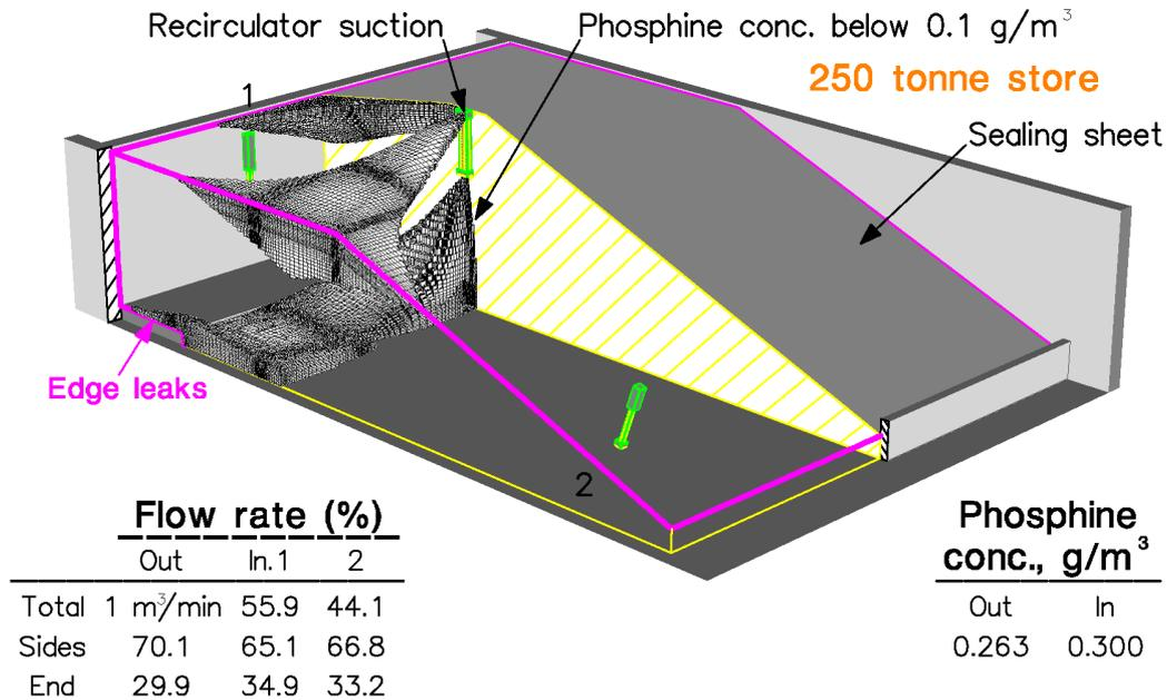
There is evidence from the experimental results that the leakage shown in Figures 12 and 13 at the sheet side was present in the tests, due to the difficulty of sealing the sheet against a corrugated wall. However, tests with a sulphur hexafluoride ( $\text{SF}_6$ ) based leak detector suggest that the edges of the sheet are generally well sealed. Also this test failed to find leakage near point G through the party wall into the next part of the store.
