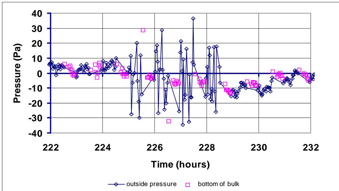
Ambient pressure fluctuations of increased amplitude during another stormy period are shown in Figure 23. There is some evidence that the amplitude of the pressure waves is less damped at the top of the bulk compared with the bottom. Both are much less than outside the sheeting which illustrates the benefit given by the sheets during windy conditions. The five outlying low pressure readings at the bottom of the bulk in the early part of this segment were caused by the multiplexer cycle.
