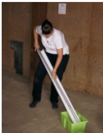
Figure 1. Multi-compartmented sampling spear.
