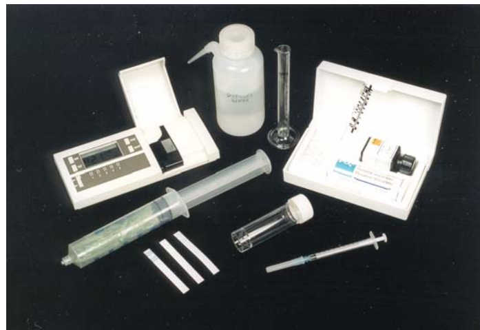
Figure 1.4 On-farm test kit for Pi analysis: RQflex2 reflectometer, Pi test strips, syringe
