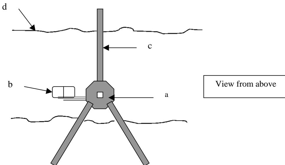
Fig. 3. Diagram of the camera jig. a) ratchet to hold vertical support for the camera; b) camera with viewing screen uppermost; c) supporting legs; d) profile wall of soil pit.
