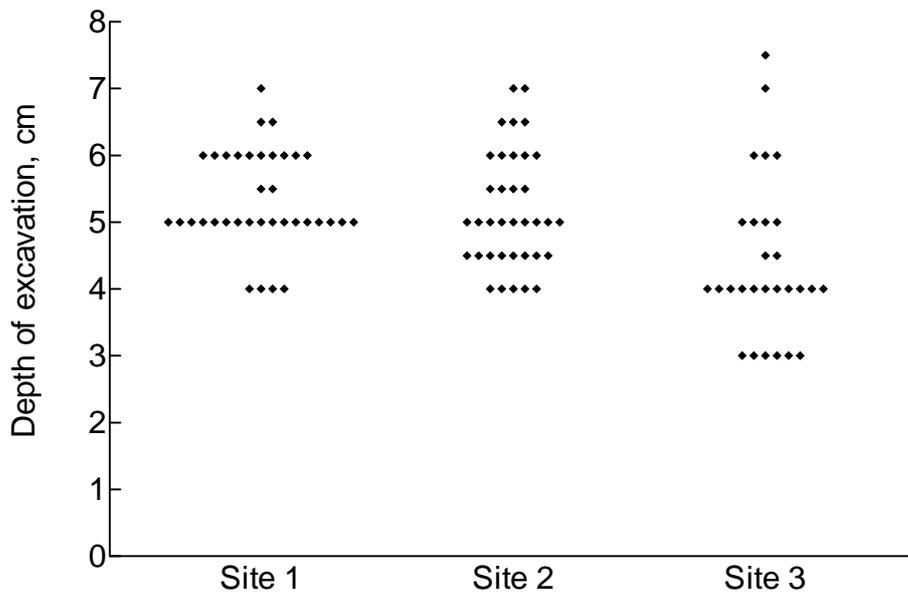
Fig. 9. Scatter diagram illustrating the extent of variation in excavation depth at each site. Each symbol represents the depth at one point in the 20 x 20 cm grid on the profile wall. Data for replicate profile walls have been pooled. Means  $\pm$  SD for the sites were: site 1,  $5.3 \pm 0.7$ ; site 2,  $5.2 \pm 0.9$ ; site 3,  $4.4 \pm 1.2$ .
