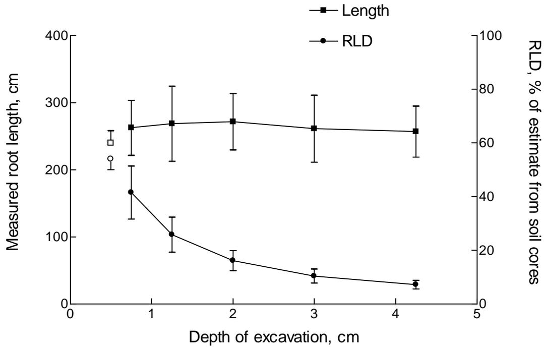
Fig. 10. Root length measured from images of the profile wall after excavating to different depths. Solid squares, root length after air-knifing; open square, root length after hand excavation; circles, estimated root length density (RLD; root length per unit volume of soil) as a percentage of that determined by soil coring (solid circles, soil excavated by air knife; open circle, soil excavated by hand). Values are means  $\pm$  SE of 4 replicate soil pits (3 in the case of hand excavation).
