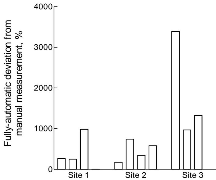
Fig. 6. Overestimation of root length by fully automatic analysis: variation between images of replicate soil pits
