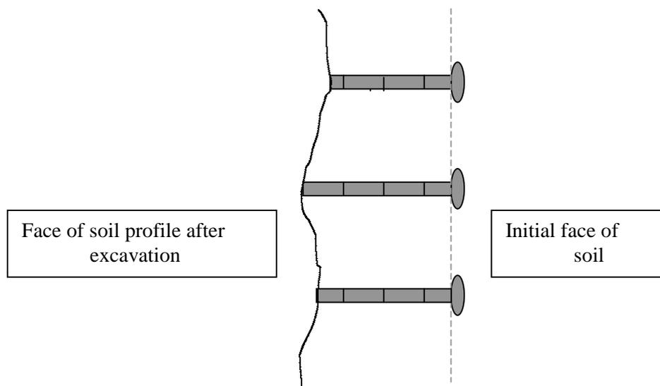
Fig. 2. Diagram of a section through the profile wall to illustrate the use of marking bolts to gauge the depth of excavation.
