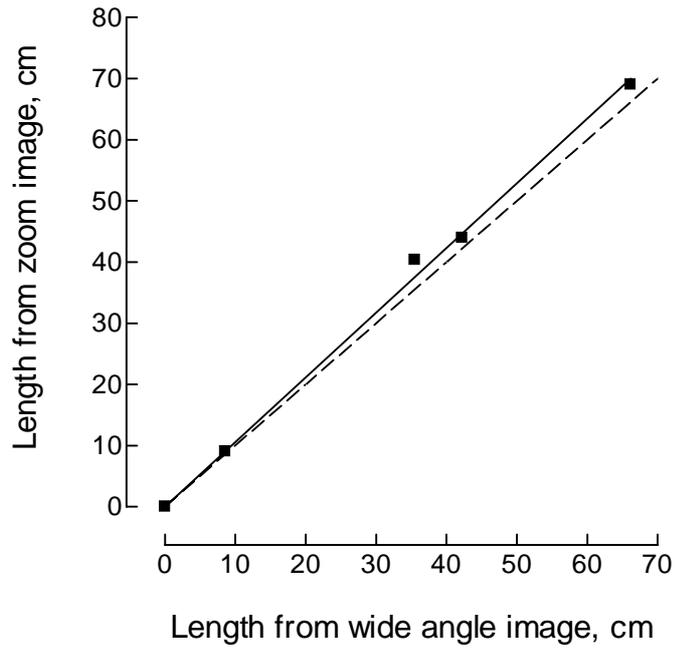
Fig. 8. Relationship between root length measured from close up (zoom) photographs of a particular zone on the profile wall and wide-angle photographs of the same zone. Solid line fitted by regression,  $y = 1.06x$ ;  $r^2 = 0.999$  (SE of slope = 0.0174). Broken line indicates 1:1 relationship.
