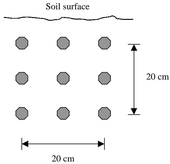
Fig. 1. Arrangement of marking bolts to form 20 x 20 cm grid on the face of the profile wall.
