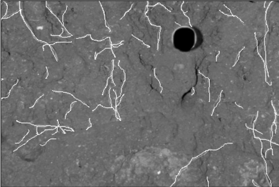
Fig. 4. Close up of one section of a profile wall image showing tracings of roots and a marking bolt 'painted out' to exclude it from the analysis.
