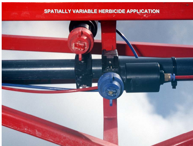
Fig. 5.1 Details of the spray boom of the PatchSpray sprayer, showing the valves that control the nozzles
