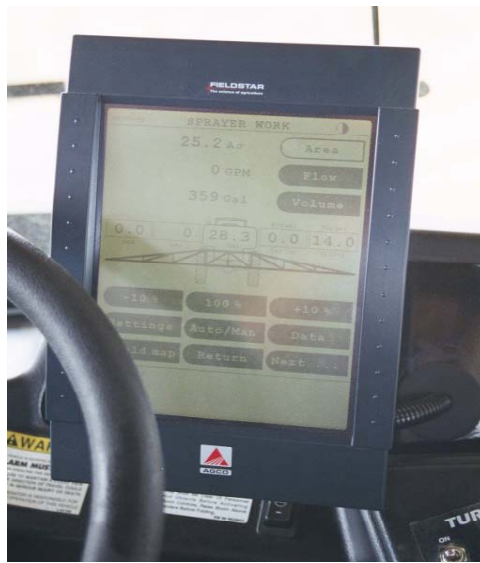
Fig. 3.2 'Fieldstar' touch-sensitive screen mounted in the 'Spra-Coupe' sprayer
