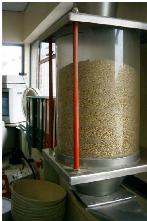
Figure 1. The collection of samples from lorry-loads of barley with a Samplex CS90
