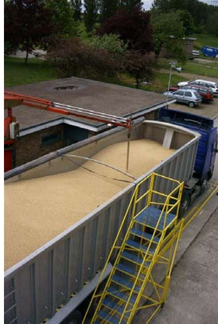
Figure 1. The collection of samples from lorry-loads of barley with a Samplex CS90
