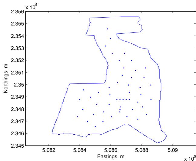
**Figure 2.6. One hundred and twenty five point sample scheme designed by minimization of  $\sigma_T^2$  for a spherical variogram with  $c_0 = 0.127$ ,  $c_1 = 1.000$  and  $a = 90.0$ .**
