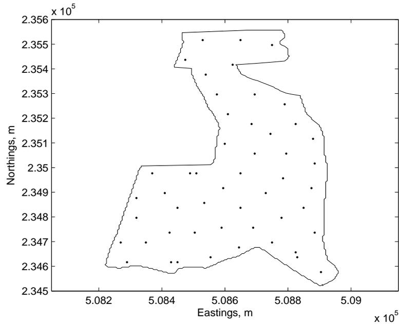
**Figure 2.4. Fifty point sample scheme designed by minimization of  $\sigma_T^2$  for a spherical variogram with  $c_0 = 0.127$ ,  $c_1 = 1.000$  and  $a = 120.0$ .**
