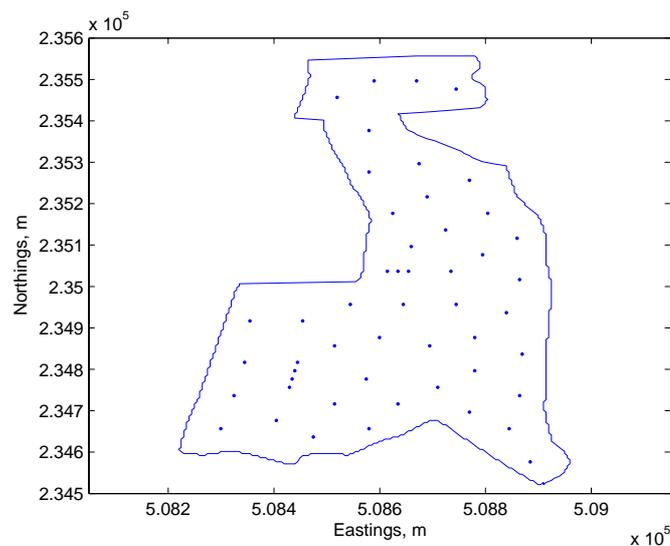
**Figure 2.5. Fifty point sample scheme designed by minimization of  $\sigma_T^2$  for a spherical variogram with  $c_0 = 0.127$ ,  $c_1 = 1.000$  and  $a = 90.0$ .**
