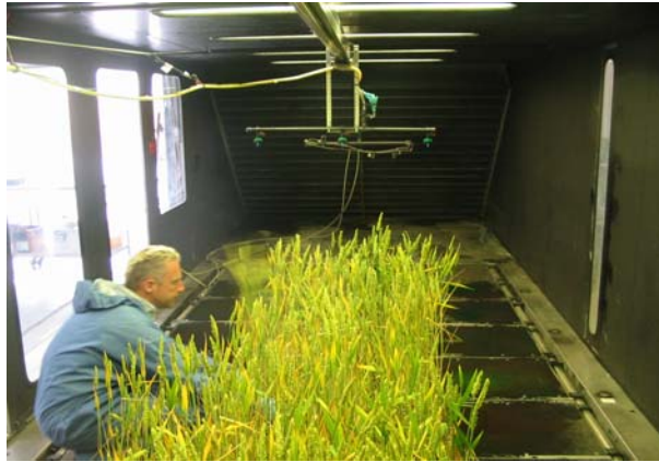
Fig. 2. Tray grown wheat crop and spray transporter in Silsoe wind tunnel
