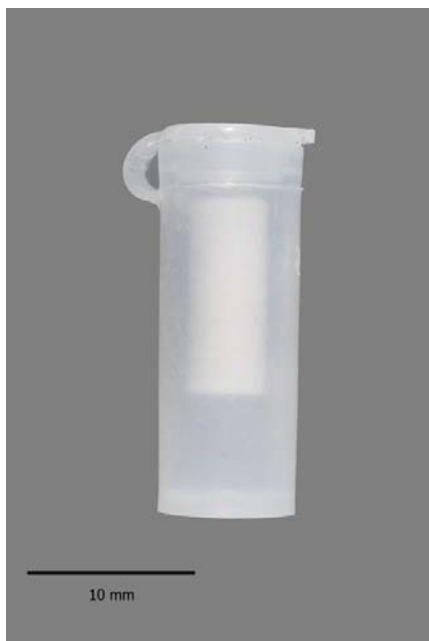
Figure 6. A vial lure containing cellulose acetate filler
