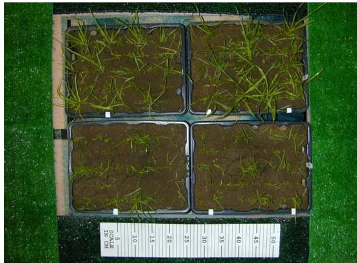
Figure 4. Trays of Italian ryegrass used for laboratory measurement of deposition on plants. Large plants (GS 20–30) are at the top, small plants (GS 11–15) at the bottom.
