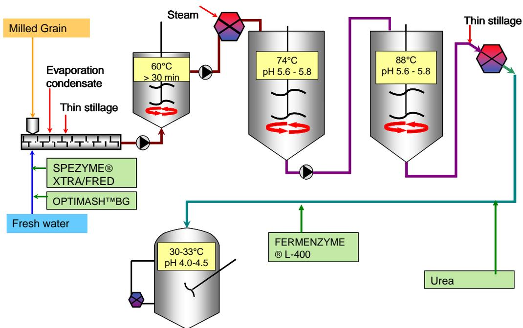
**Figure 1 Schematic diagram of typical bioethanol process with points indicated for addition of enzymes and urea (green boxes). Image courtesy of Genencor.**
