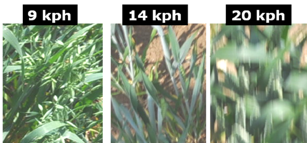
Figure 14. Images captured at tractor speeds of 9, 14 and 20 km h -1 (kph) using the Nikon D90 camera mounted on an extension piece attached to the roof of tractor cab (Figure 1A).
