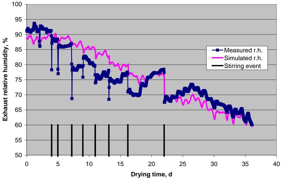
**Figure 32.** Relative humidity of exhaust air from stirred bin, Bin 3, versus time. Measured and simulated traces are shown.
