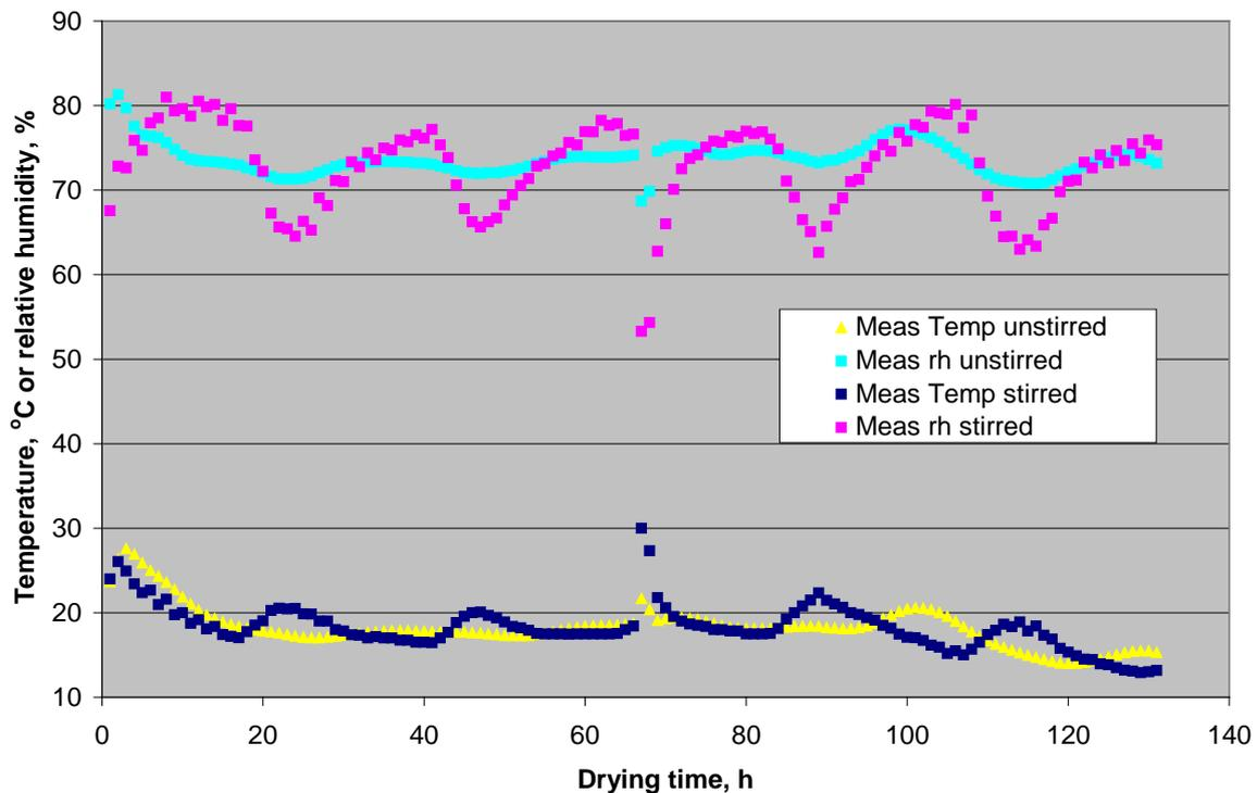
**Figure 37.** Measured exhaust conditions of temperature and relative humidity for the stirred and static blocks of the farm store.
