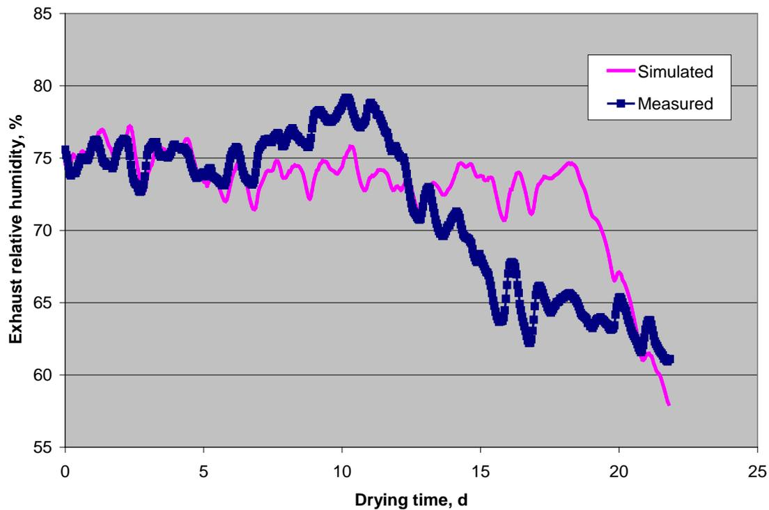
**Figure 33.** Relative humidity of exhaust air from the static bin, Bin 4, versus time. Measured and simulated traces are shown.
