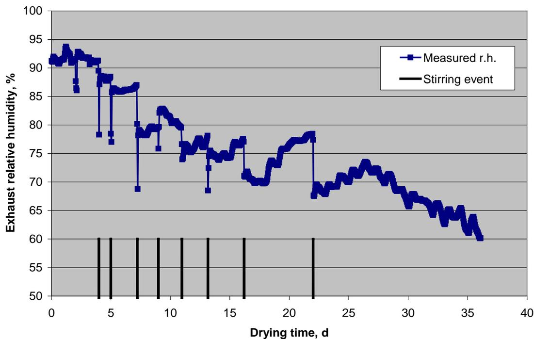
**Figure 22.** Relative humidity of air exhausting from the stirred bin, Bin 3, versus drying time.
