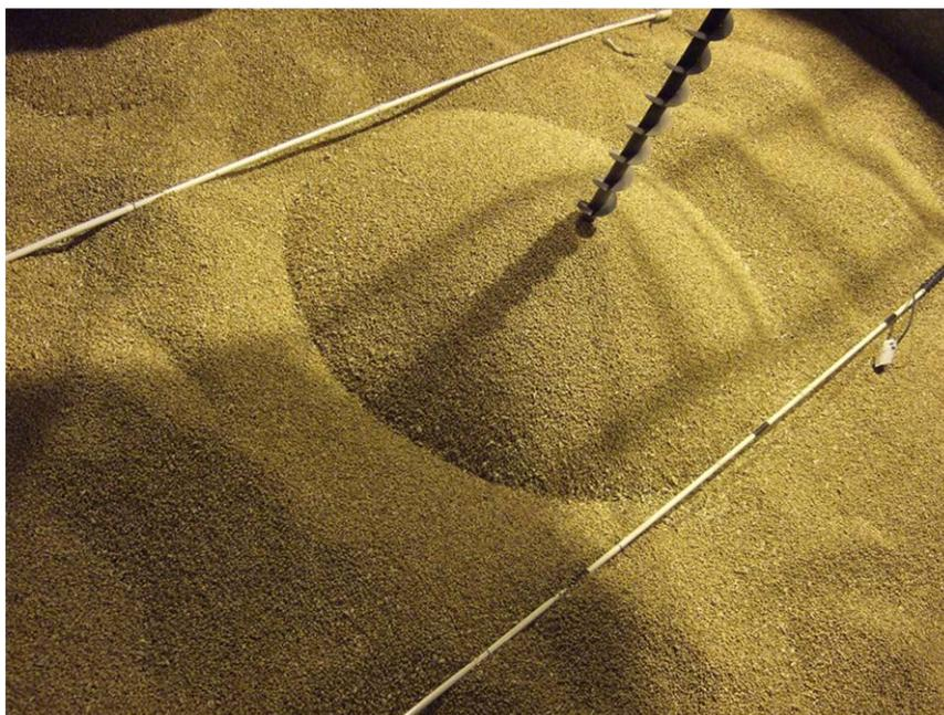
**Figure 10.** Grain cone formed by running the auger
