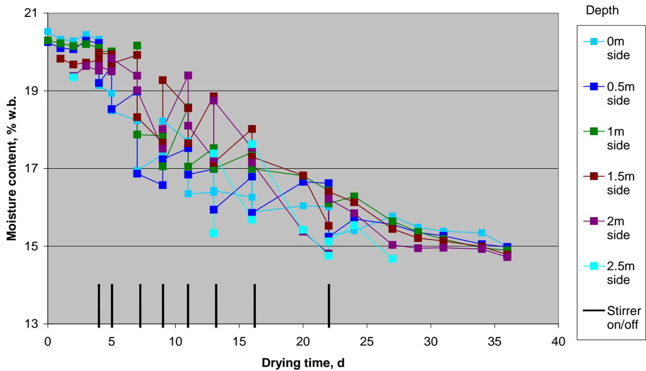
**Figure 19.** Moisture content versus drying time. Samples from side of stirred bin, Bin 3, before and after stirring.
