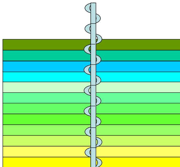
**Figure 3.** Bed after lateral redistribution in the simulation, the colours illustrating the differing proportions in each layer of mixed grain from the circulating zone and undisturbed grain.
