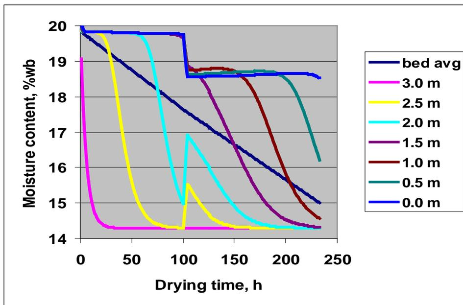
**Figure 5.** Moisture content at 7 depth locations and average moisture content versus time in a bed 3m deep stirred once at 100h.
