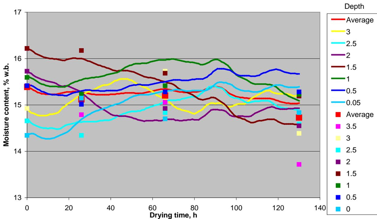
**Figure 42.** Experimental m.c. data (points) and simulated m.c. (lines) for the static block of the farm store.
