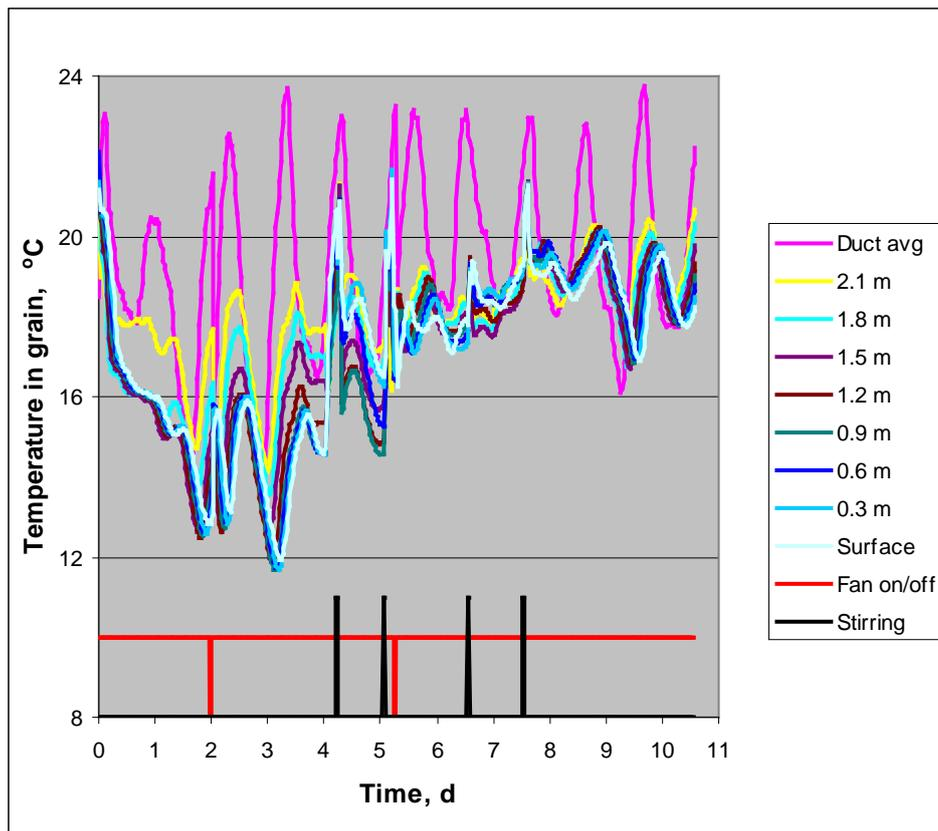
**Figure 15.** Temperatures at centre of bin versus time
