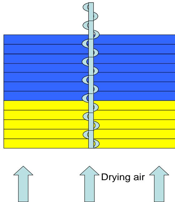
**Figure 1.** Schematic of a partly dried bed of grain showing airflow, stirring auger, grain already dried (yellow) and yet to be dried (blue).
