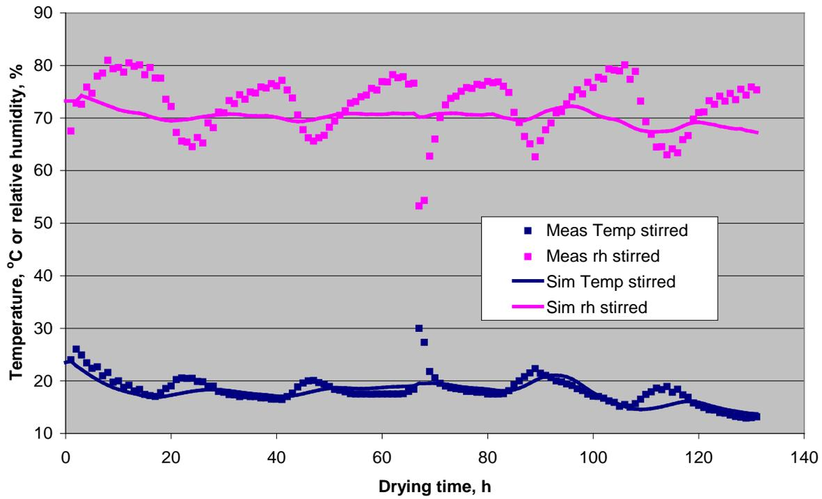
**Figure 38.** Measured and simulated exhaust conditions of temperature and relative humidity for the stirred block of the farm store.
