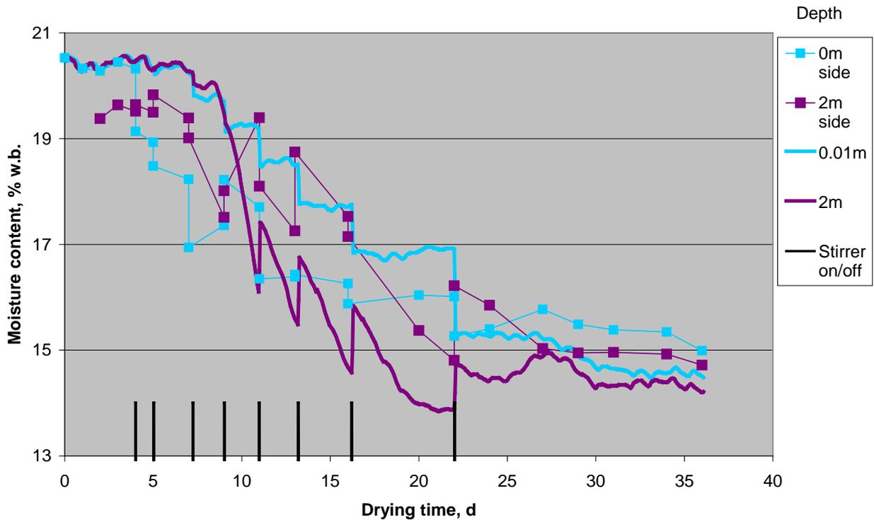
**Figure 27.** Progress of moisture content at 0 and 2m depth at side of stirred bin, Bin 3. Experiment (points and thin lines) vs simulation (thick lines). Stirring events - spikes on time axis.
