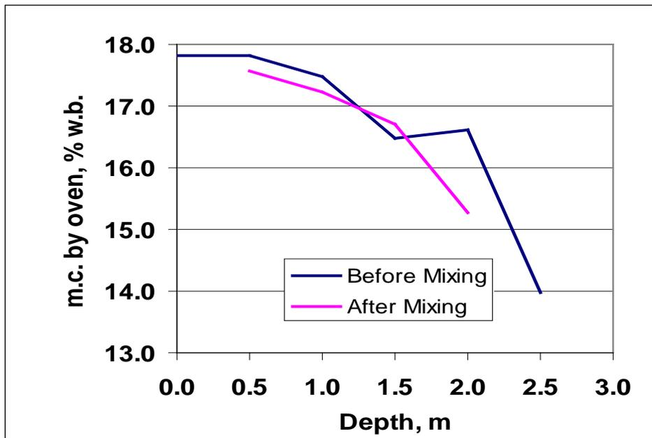
**Figure 11.** Effect of 20 min stirring on moisture content profile at 0.2m from auger axis.
