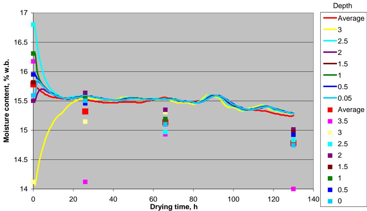
**Figure 41.** Experimental m.c. data (points) and simulated m.c. (lines) for the stirred block of the farm store.
