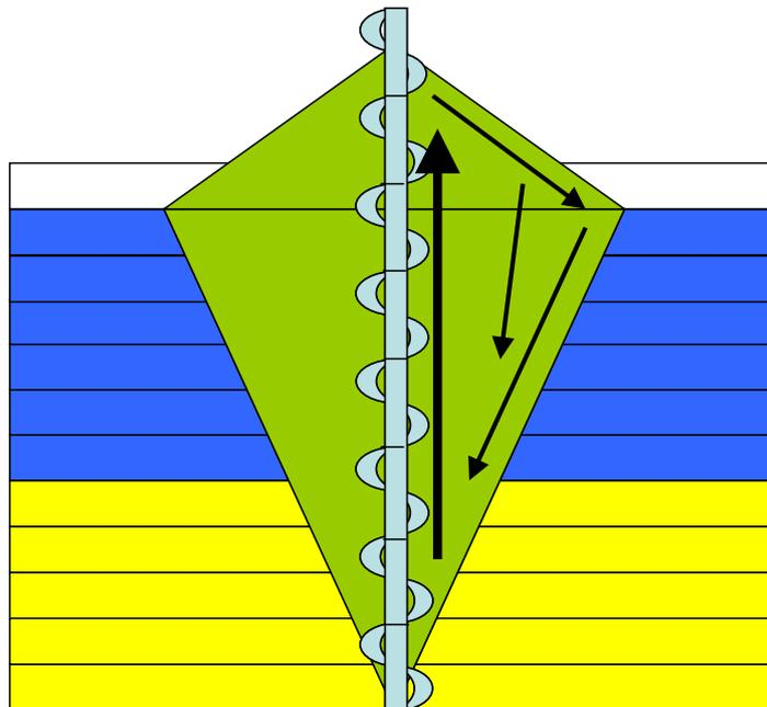
**Figure 2.** Circulation zone formed by auger (green), with arrows indicating grain flow direction and speed. The rest of the bed is undisturbed except that the level beyond the cone has fallen, shown by the white 'layer' of displaced grain.
