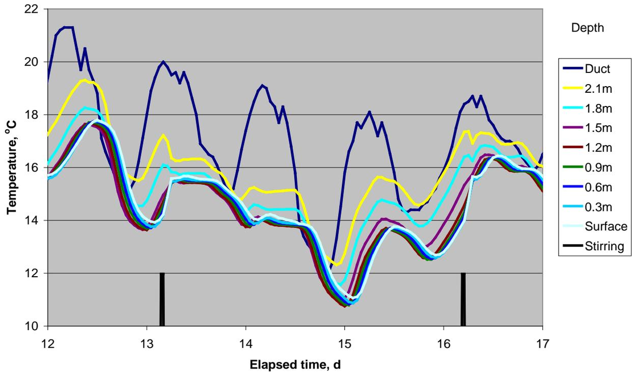
**Figure 31.** Simulated temperatures at centre of stirred bin, Bin 3.
