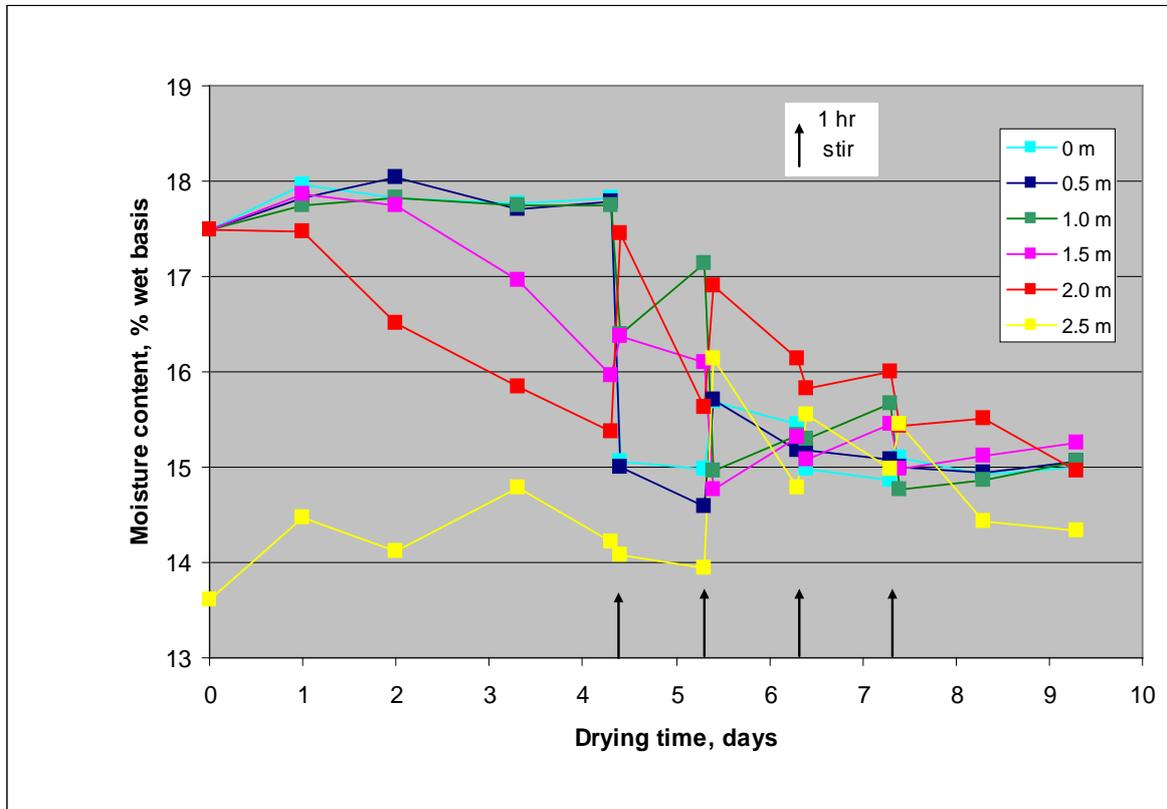
**Figure 13.** Moisture content versus time at 6 depths at edge of bin showing four times when bin was stirred
