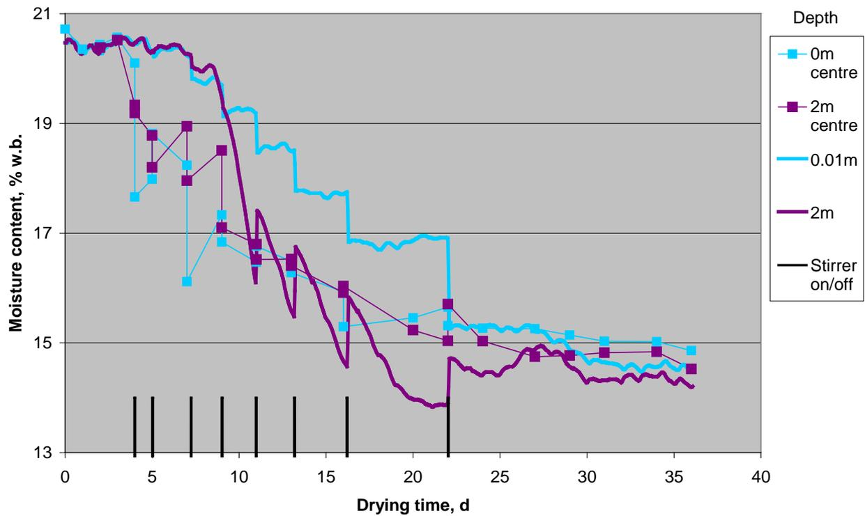
**Figure 25.** Progress of moisture content at 0 and 2m depth at centre of stirred bin, Bin 3. Experiment (points and thin lines) vs simulation (thick lines). Stirring events - spikes on time axis.
