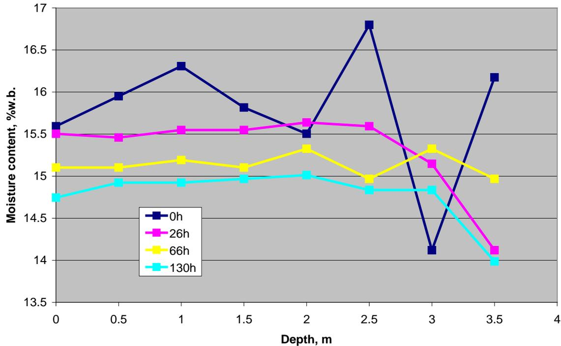
**Figure 35.** Stirred bed. Moisture content in farm store at 8 depths at each of 4 drying times.
