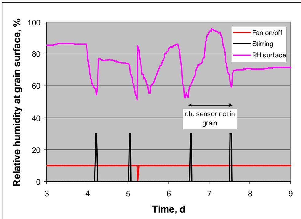
**Figure 16.** Effect of four stirring events on relative humidity at bed surface.
