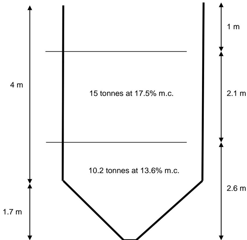
**Figure 8.** Bin 3 after loading and levelling.
