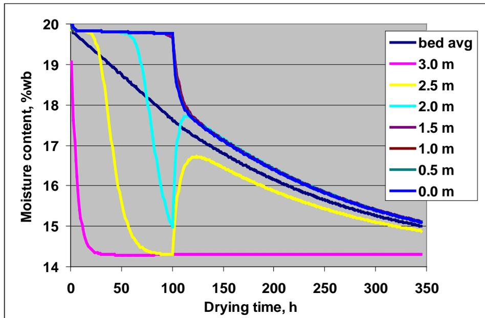
**Figure 6.** Moisture content at 7 depth locations and average moisture content versus time in a bed 3m deep stirred continuously from 100h.
