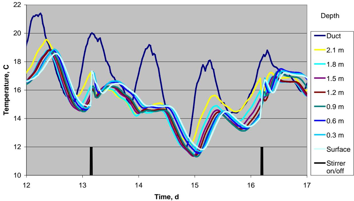
**Figure 30.** Measured temperatures at centre of stirred bin, Bin 3.
