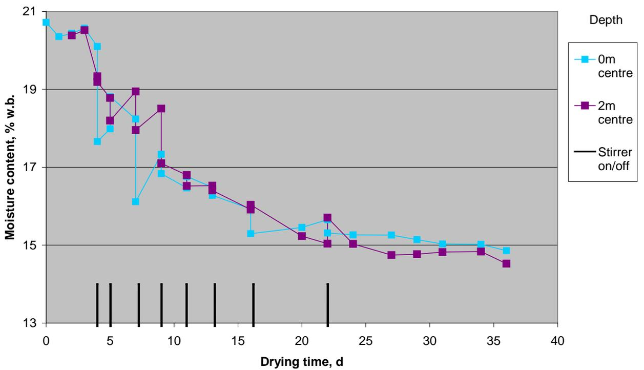
**Figure 18.** Moisture content versus drying time. Samples taken from centre of stirred bin, Bin 3, before and after stirring. For clarity, only data from 0 and 2m depth are shown.
