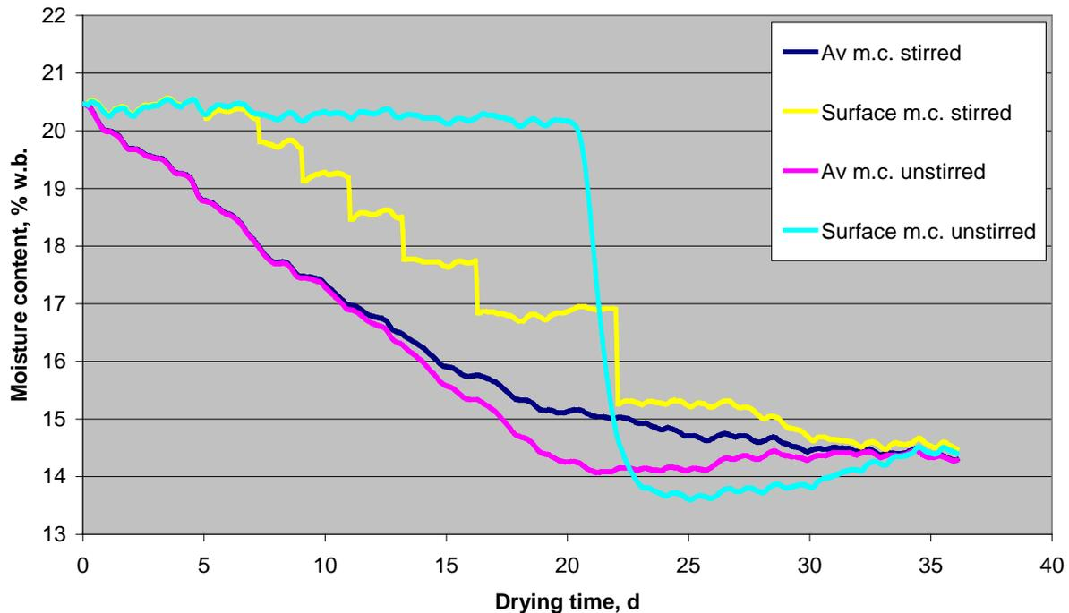
**Figure 34.** Simulated average and surface m.c. versus time, for the stirred bin and the static bin with same starting condition.
