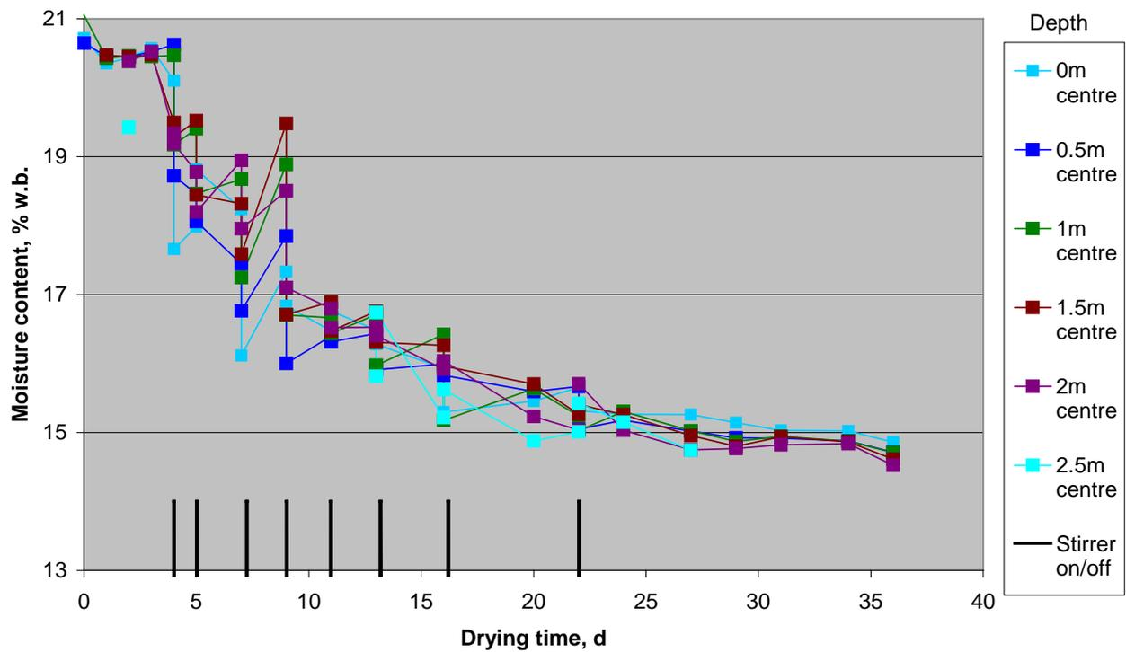
**Figure 17.** Moisture content versus drying time. Samples from centre of stirred bin, Bin 3, before and after stirring. Stirring events are shown by spikes on time axis. Points are joined by lines to show which sample was before and which after stirring.
