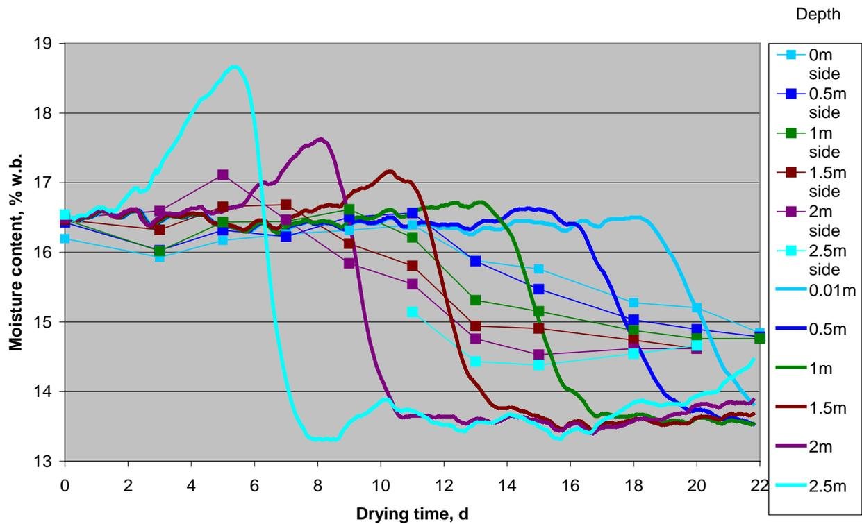
**Figure 29.** Progress of moisture content at side of the static bin, Bin 4. Experiment (points and thin lines) vs simulation (thick lines).
