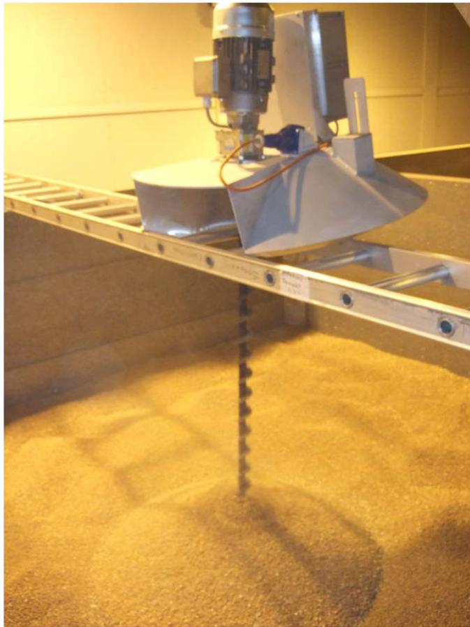
**Figure 9.** Single auger stirrer unit secured across the bin.
