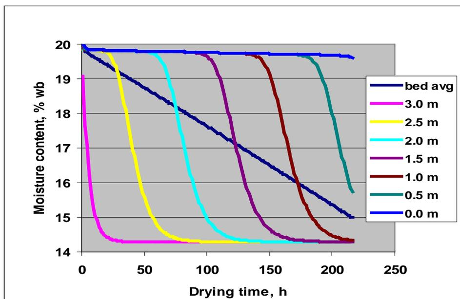
**Figure 4.** Moisture content at 7 depth locations and average moisture content versus time in a static bed 3m deep.
