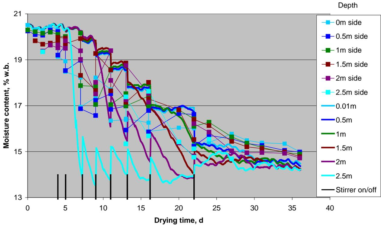
**Figure 26.** Progress of moisture content at side of stirred bin, Bin 3. Experiment (points and thin lines) vs simulation (thick lines). Stirring events - spikes on time axis.
