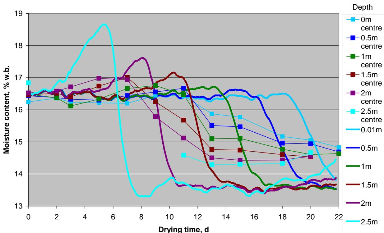
**Figure 28.** Progress of moisture content at centre of the static bin, Bin 4. Experiment (points and thin lines) vs simulation (thick lines).
