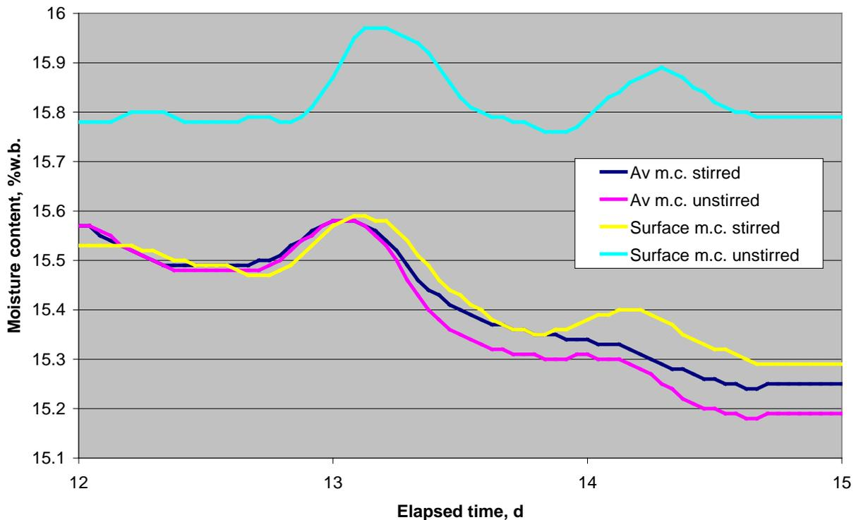
**Figure 43.** Progress of average bed and bed surface m.c. by simulation of stirred block of farm store, and of static block at same initial conditions.
