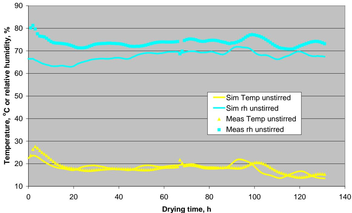
**Figure 39.** Measured and simulated exhaust conditions of temperature and relative humidity for the static block of the farm store.
