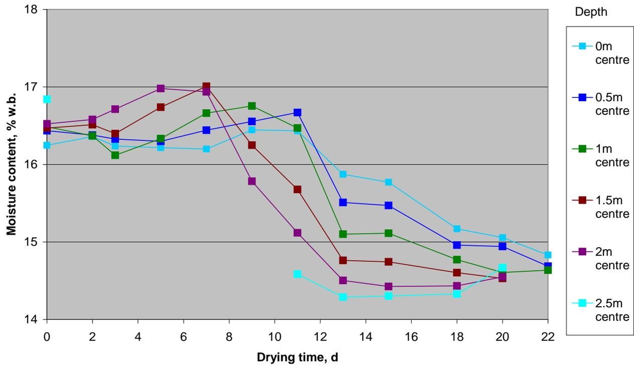
Figure 20. Moisture content versus drying time. Samples from centre of the static bin, Bin 4.
