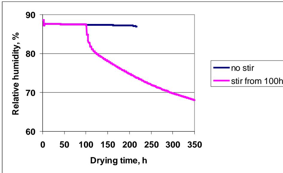
**Figure 7.** Exhaust air r.h. from static bed and from bed stirred from 100h, versus time.
