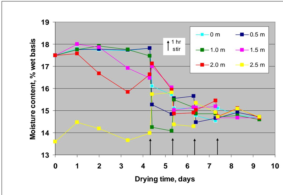
**Figure 12.** Moisture content versus time at 6 depths at centre of bin showing four times when bin was stirred.
