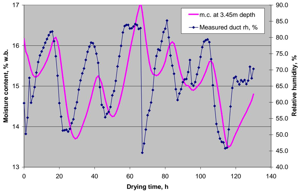
**Figure 40.** Relative humidity of air in the inlet duct and m.c. by simulation close to this depth.
