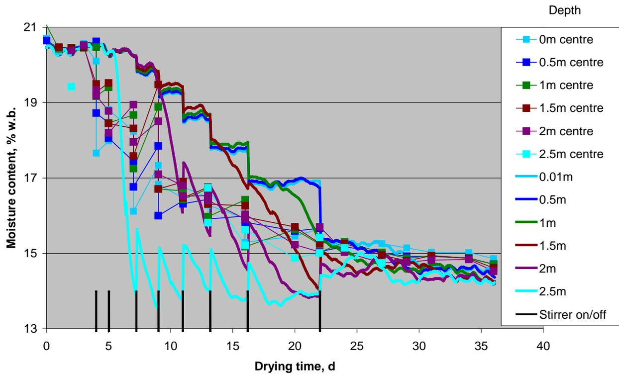
**Figure 24.** Progress of moisture content at centre of stirred bin, Bin 3. Experiment (points and thin lines) vs simulation (thick lines). Stirring events - spikes on time axis.
