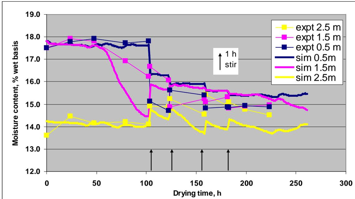
**Figure 14.** Progress of moisture content with time during drying, experiment versus simulation.
