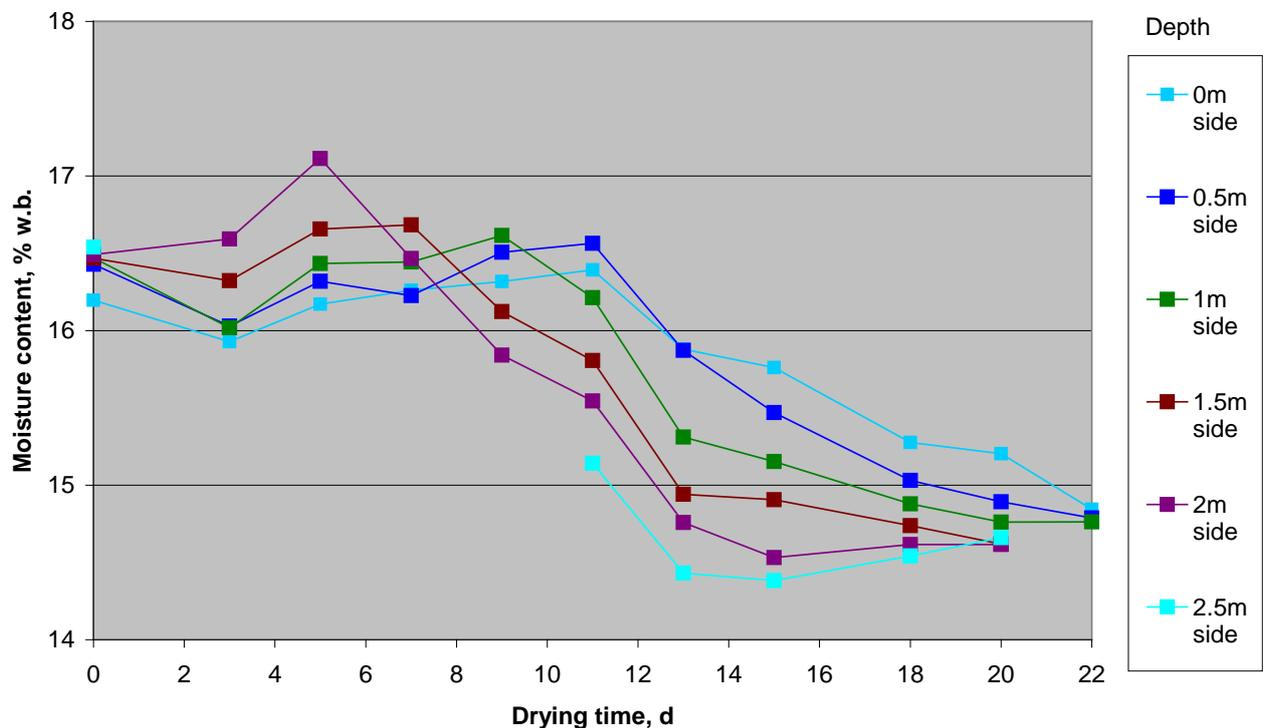
Figure 21. Moisture content versus drying time. Samples from side of the static bin, Bin 4.
