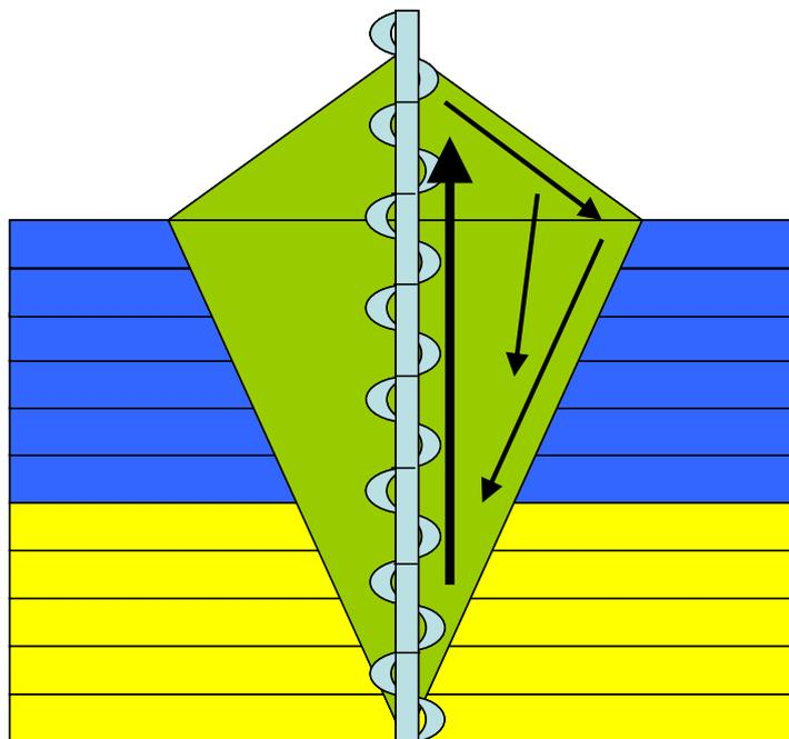
**Figure 1.** Circulation zone formed by auger (green), with arrows indicating grain flow direction and speed.
