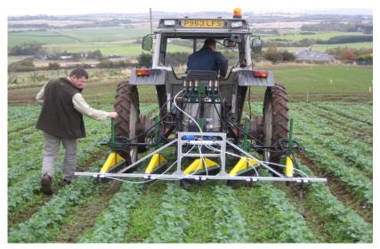
Figure 67. Test rig in action at SAC site in year one of the project.
