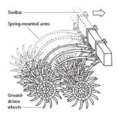
The rotary hoe (Figure 3) referred to in the following section is ground driven, it has one or more sets of vertical star shaped wheels mounted on a horizontal axis. The wheels are 21 inches in diameter with 16 teeth. Speed of work is 15–18 km/hr. They work at 2–3 cm depth. The machine works over the whole field area like the tine weeder.
