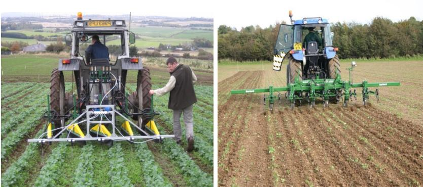
SAC test rig, year using CDA sprayer ORC using inter-row cultivator
