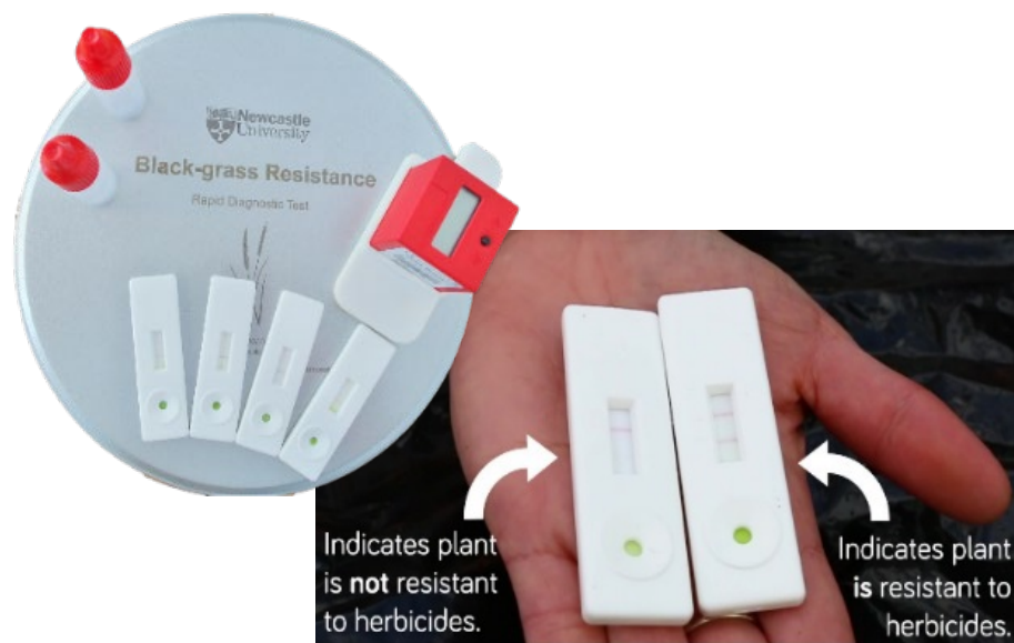
Figure 6. On-farm diagnostic test for MHR in blackgrass
