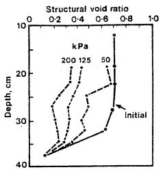
Change in pore space (void ratio) with depth, when a tractor tyre with different inflation pressures passes over a clay soil with a dry surface (0-7 cm.) overlying a wet sub-surface.
