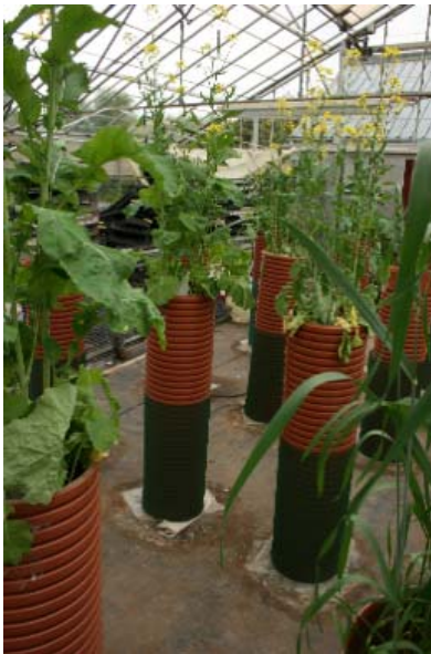
Figure 2. The lysimeters with oilseed rape and wheat plants at the day of harvest. The green mesh shading the mini crops during growth was slid down.
