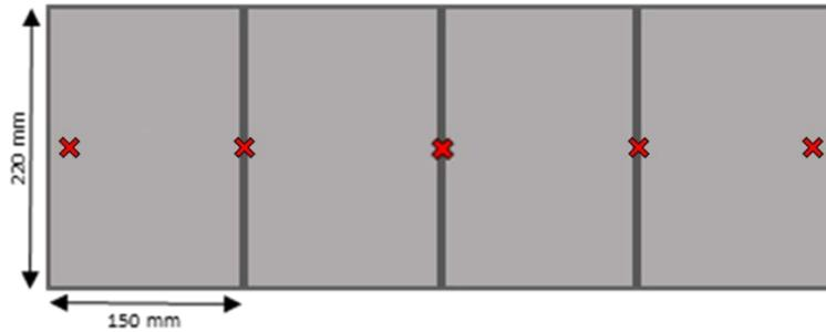
Figure 3. Showing the dimensions and arrangement of one of the sets of four trays along with the positions of the five data loggers, illustrated by the red crosses, used to measure the temperature gradient.
