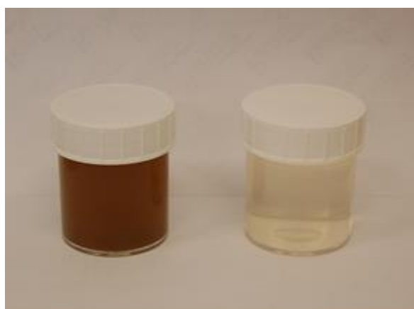
Figure 7-2 Drainage water samples 10 days after slurry application to grassland at Faringdon in March 2008: slurry treated (left) and untreated (right)
