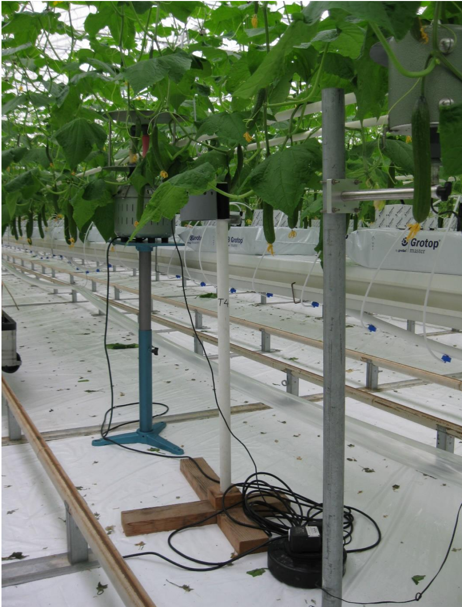
Figure 4. Three air samplers (left to right - single cyclone, MTIST and multi-vial cyclone) set at a sampling height of 1 m in a UK commercial cucumber crop.
