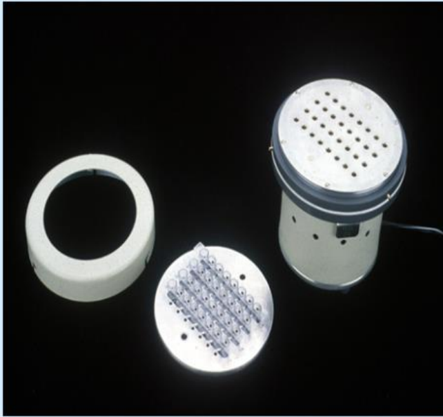
Figure 5. Personal MTIST air sampler with four, eight well microtitre strips
