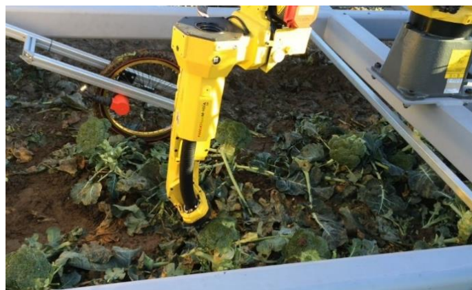
Robotic arm pointing to correct sized broccoli head during field trials.
