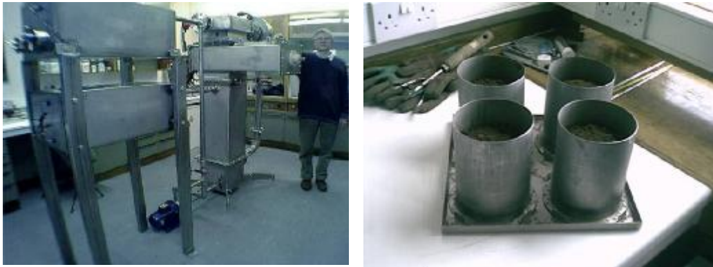
Figure 4. A) Laboratory prototype steamer, B) The four replicate cylinders used in the prototype, each of which holds 1 litre of soil. Soils were spiked with test organism prior to steaming, then survival was assessed
