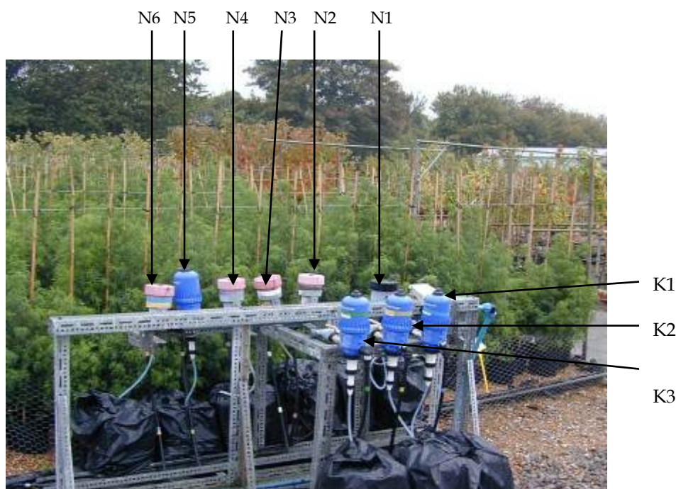
Figure 16. Structure of the dosatron arrangement supplying different concentrations of nitrogen to the plants in the N-experiment
