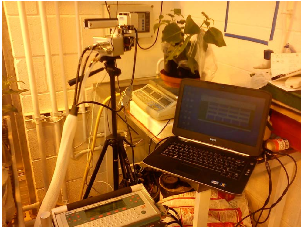
Fig.1. The LICOR LI-6400XT Photosynthesis System used to record various physiological variables from plants in the study.
