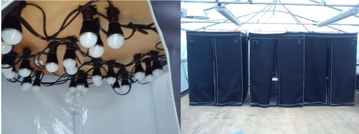
Fig.5. The environment chambers used for the red:far red experiment, equipped with high-intensity variable LED arrays used to manipulate the red:far red ratio.
