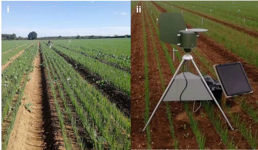
i) Trial layout, ii) Burkhardt spore trap in trial area.
