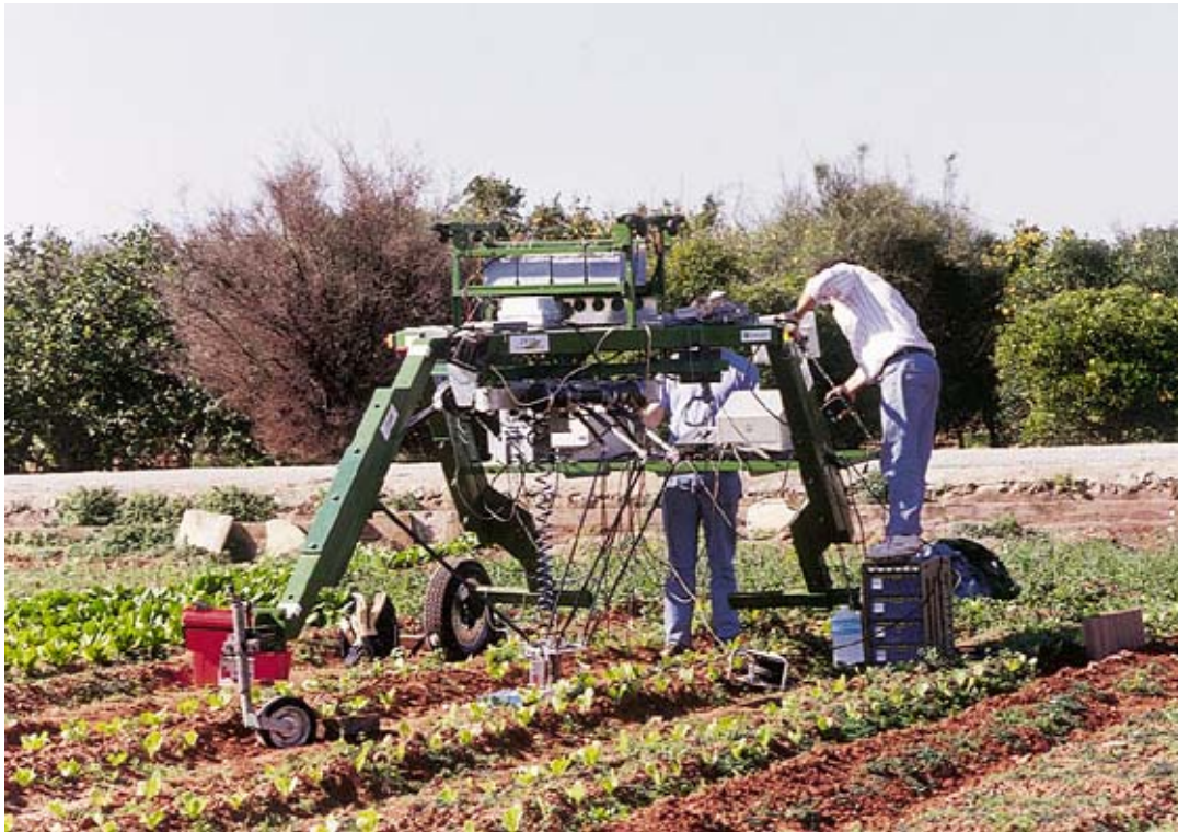
Fig. 4. Selective electric weeding using a mobile robot.
