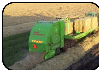
Poly + straw laying
