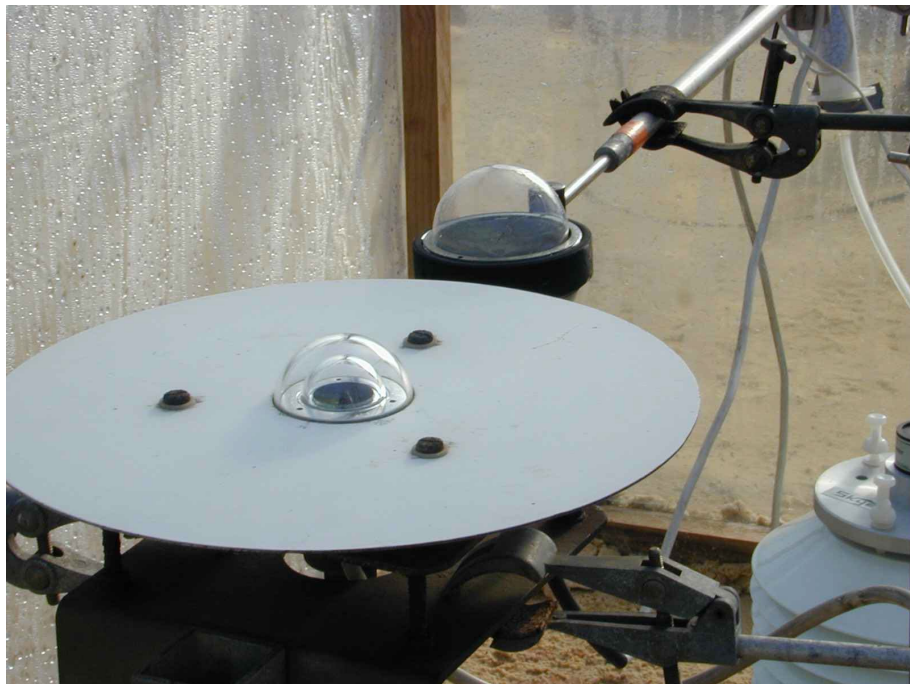
Plate 16. The solarimeter (at the front, with a double glass dome) and net radiometer (at the back with a single inflated polythene dome) inside a E3 type enclosure for thermal radiation measurements.
