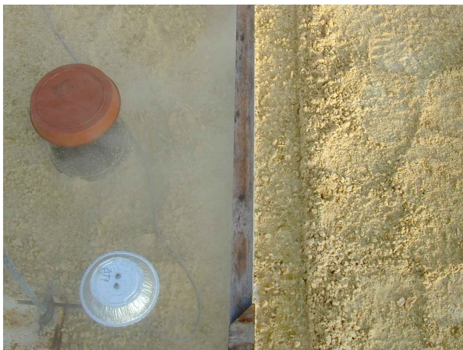
Plate 14. View from above a 30cm polythene wall which is retaining a layer of fine droplet ultrasonic fog in a small fog 'pen'. The inverted pot and saucer make an effective distributor of the fog, which is fed in through a pipe buried in the sand. The aluminium dish is a reflective 'hat' over a psychrometer used to monitor the effect of the fog on humidity.
