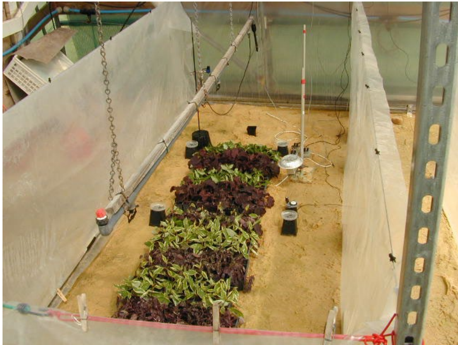
Plate 5. The open mist bed with surrounding polythene curtain to reduce currents of dry air from the surrounding non-misted areas. Note the plastic dishes for measuring wetting and the reflective 'hat' on the psychrometer to minimise the effect of radiation on measurements of temperature and humidity.
