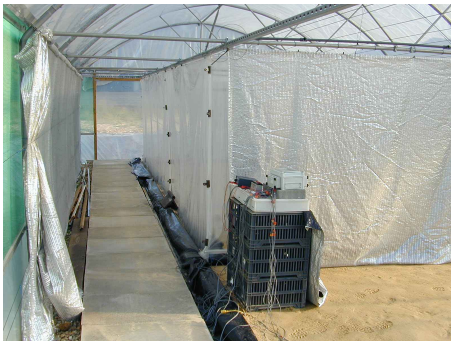
Plate 1. Outside of the large-scale enclosed mist chamber, with data logging equipment in the foreground. Notice that the roof and gable are shaded externally while vertical shade walls are inside the polyhouse (end wall not yet covered at the time of this photo).
