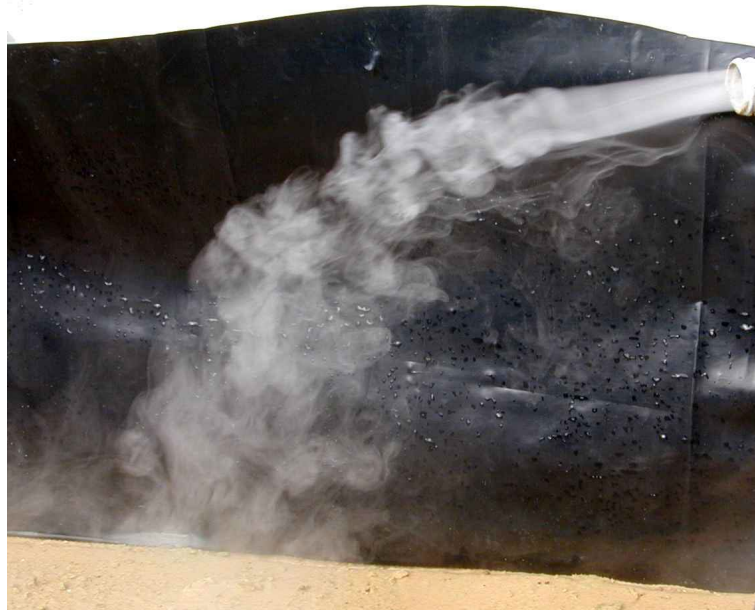
Plate 13. A slow moving stream of air carrying very fine droplet fog (generated ultrasonically) falls gently downward. If air currents are reduced sufficiently the fog can be contained as a blanket around cuttings.
