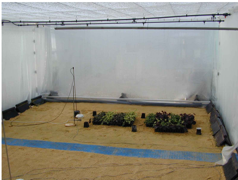
Plate 2. Inside the large-scale enclosed mist system. Transparent plastic dishes on stands amongst the cutting are for monitoring water deposition.
