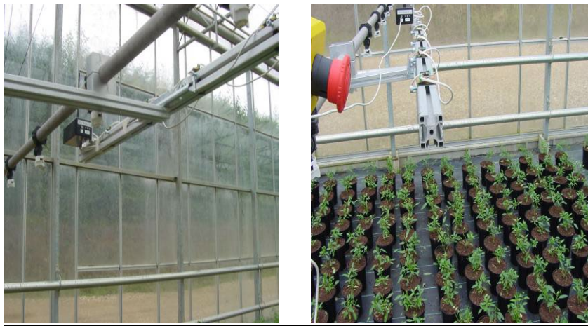
Figure 7.8. The thermopile system with remote monitoring mounted on a gantry watering system.
