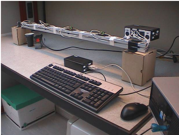
Figure 7.3. The Gantry test rig with wireless connection.
