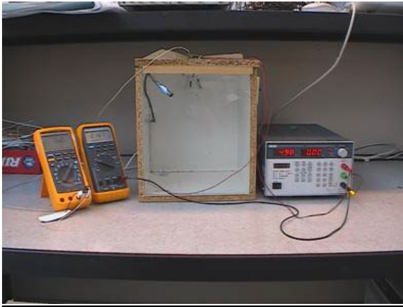
Figure 7.2: Thermistor under testing for uniformity.
