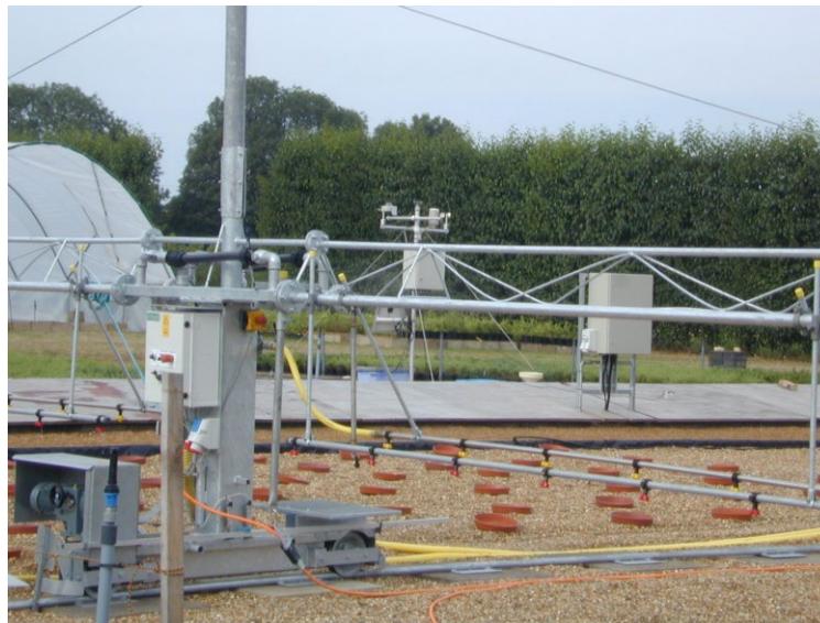
Figure 2. Overhead irrigation gantry on the EMWC
