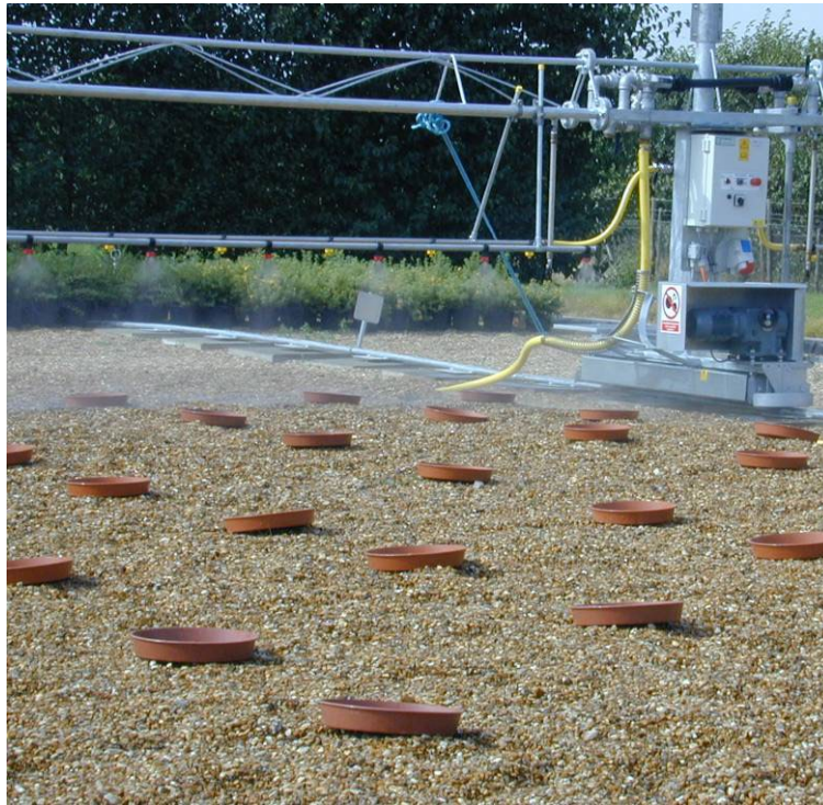
Figure 3. Capturing irrigation water in saucers to determine application rate and uniformity of water distribution
