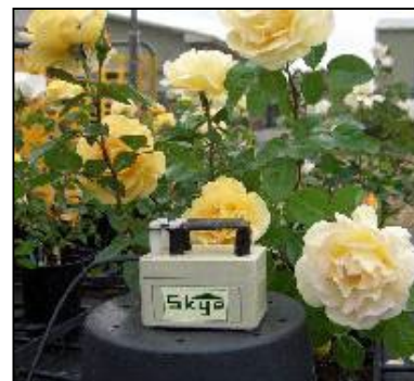
Figure 12. The Evaposensor used to estimate daily evaporative demand for use in irrigation scheduling during the Rosa RDI experiment in 2008.
