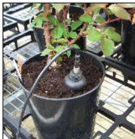
Figure 18. A SM200 soil moisture probe inserted into a containerised rose in a shelf-life test at EMR in 2009. Throughout the test, soil moisture sensing probes were used to trigger irrigation automatically to maintain the appropriate soil moisture contents in the 'wet' and 'dry' regimes.
