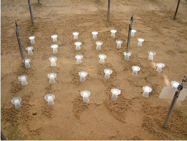
Photo 3. Testing mist distribution uniformity at New Place Nurseries, September 2007
