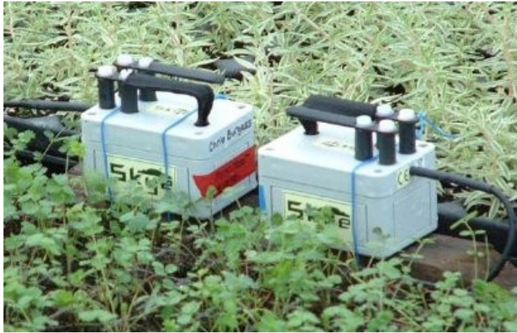
Photo GS1. Mist control and monitoring Evaposensors. Supported above cuttings to avoid shading of wet and dry 'leaves'
