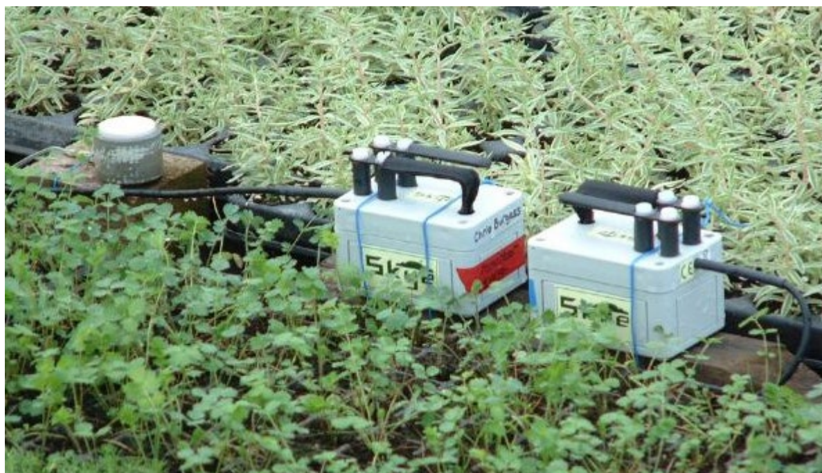
Photo 2. One Evaposensor linked to Nobel or ETS interface to control mist burst frequency and the other Evaposensor connected to logger to monitor environment achieved. PAR quantum sensor to record light levels also shown.
