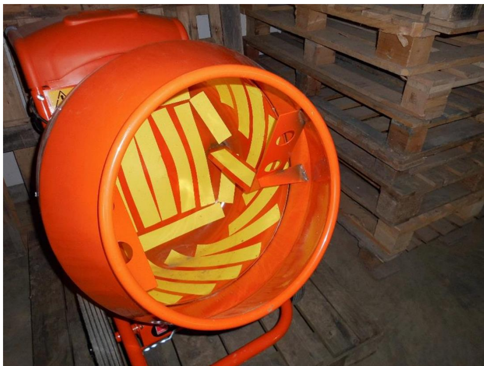
Figure 1. Cement mixer used for assessing skinset
