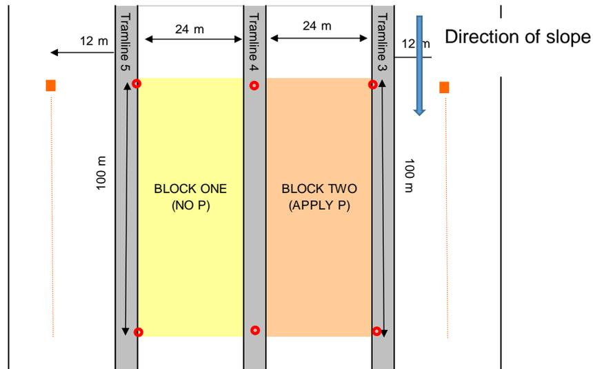
Figure 7.4. Plan of incidental run-off site: block 1 ( $P\ 17\ \text{mg}\ \text{L}^{-1}$ ) and block 2 ( $P\ 65\ \text{mg}\ \text{L}^{-1}$ ).
