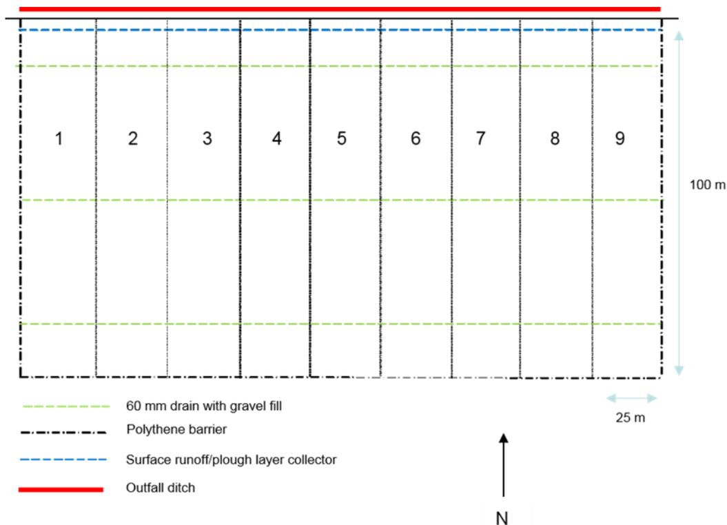
Figure 7.3. Plan of Cockle Park hydrologically isolated drainage plots
