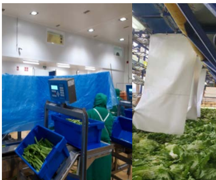
Figure 4. Examples of methods used to screen workers with plastic sheeting. Other methods could include solid Plexiglas screens
